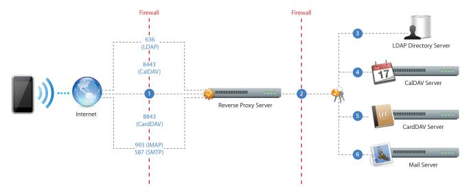
This example shows how iPhone connects to a typical IMAP, LDAP, CalDAV and CardDAV deployment.
